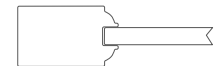
FLAT PANEL OVOLO (6000 FP SERIES) PON, RAD, KPN, PRM, OAK, POP, FIR, MHG
